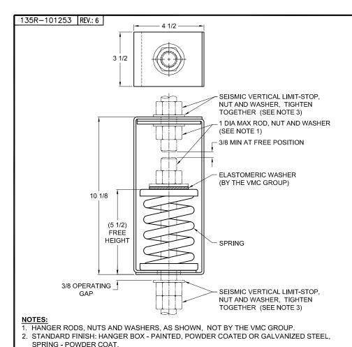
3. SEISMIC VERTICAL LIMIT-STOP REQUIRED FOR SEISMIC APPLICATIONS. NOT BY THE VMC GROUP. INSTALL WASHER .134 THK, MIN. X 2 O.D. MIN WITH REQUIRED INSIDE DIAMETER TO ACCOMMODATE ROD SIZE IN USE. THIS CAN BE ACCOMPLISHED BY USING A SINGLE WASHER OR BY STACKING NOT MORE
